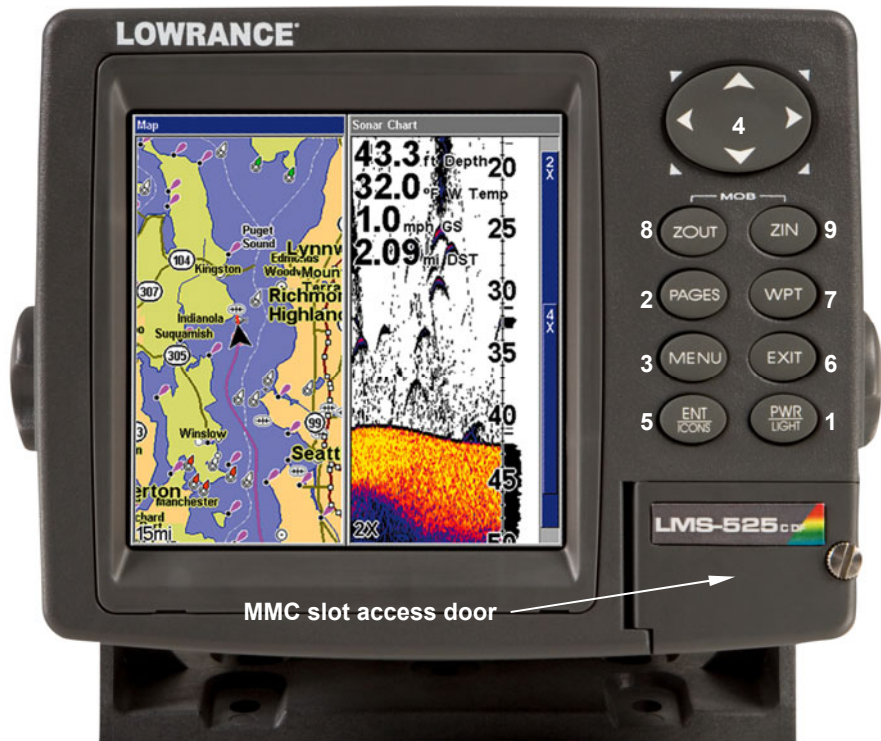
LMS-525cDF sonar/GPS unit, front view, showing map with sonar split screen, keyboard and access door for the MMC slot.
